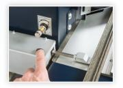
Width Measurement Device automatically measures moulding width and is temporary stored for running the job.
