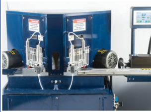
Precision machined cast table, saw head, pivot assemblies and motor bases
