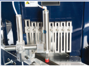
Pneumatic Hold Down Part Clamping Mechanism
