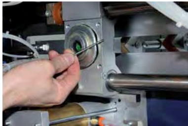
Replace the external flange seal.
