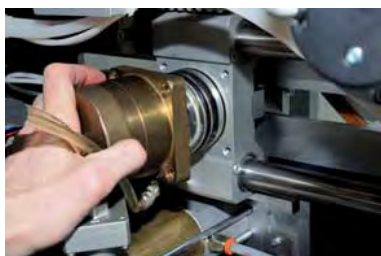
Lubricate and reinstall the cylinder.
