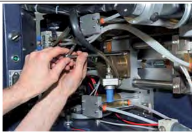
Remove the screws which hold the pneumatic cylinder in place.
