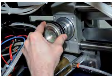
Lubricate and reinstall the piston.
