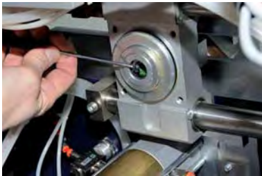
Replace the internal flange seal.
