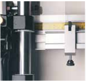
Production stops for repeatable cutting
