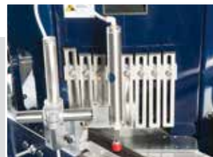
Pneumatic hold down clamping mechanism
