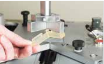
Interchangeable clamping pads
