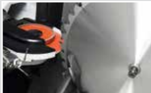
Machining the tooth face during sharpening process
