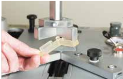
Easy field replacement enables a quick change to a different clamping pad depending on joining applications
