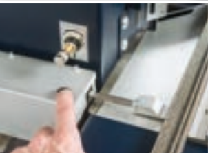
WIDTH MEASUREMENT DEVICE AUTOMATICALLY MEASURES MOULDING WIDTH AND IS TEMPORARILY STORED FOR RUNNING THE JOB.
