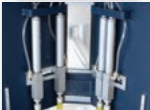
INSIDE CABINET VIEW OF PNEUMATIC HOLD DOWN CLAMPS
