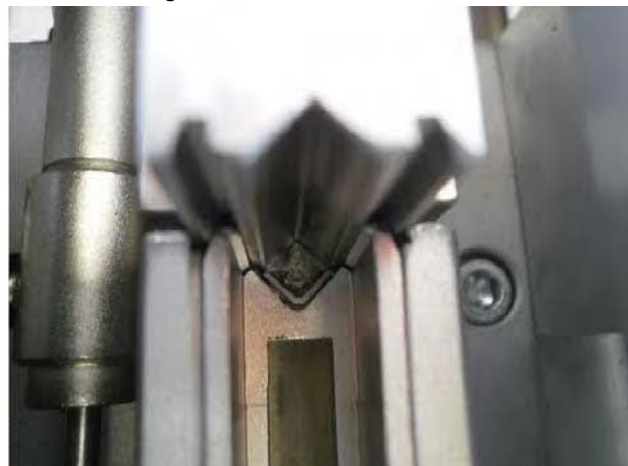
6) Check the V-nail magazine and the L support are perfectly aligned
