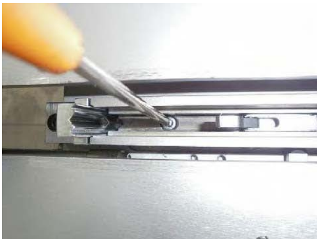
5) Bring the magazine near the L support by loosening the two M magazine locking screws
