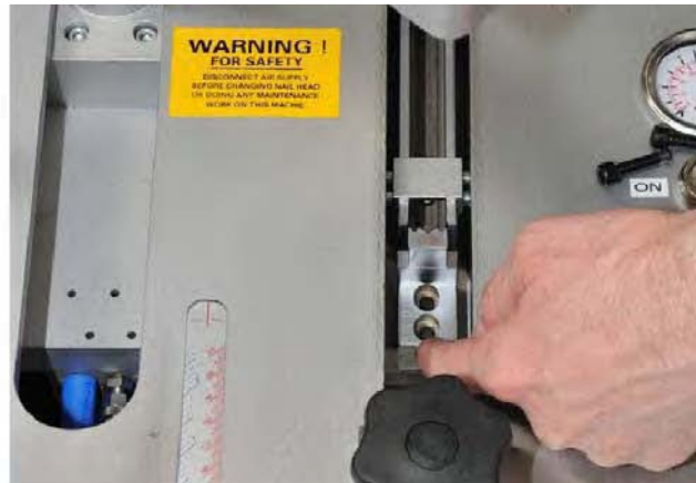
4) With the driver up, bring the L support near the driver and tighten the screws
