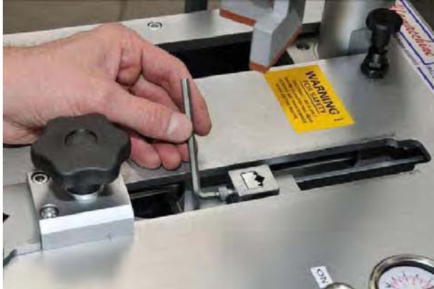
1) Loosen the 5 mm Allen screw that fixes the nail head in place
