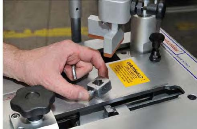
2) Remove the nail head
