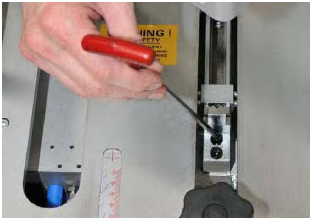
3) Loosen the screws that fix the L support
