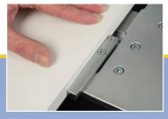
Dual position fencing slides left and right for securing the trim material during joining process
