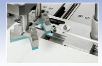
Spacer blocks are used for creating off-set joints for decorative appearance - Spacer sizes: 1", 1/2" and 1/4"
