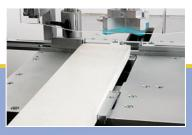
To set proper joining line, position trim in center of V-Nail head and then slide dual position fencing to secure it
