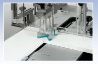
Double Hydraulic Clamp is used to secure the trim pieces during joining process
