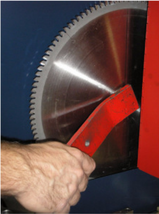
Removing the Flange Nut
