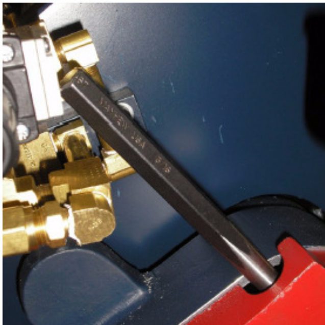
Inserting Pin into Spindle Shaft
