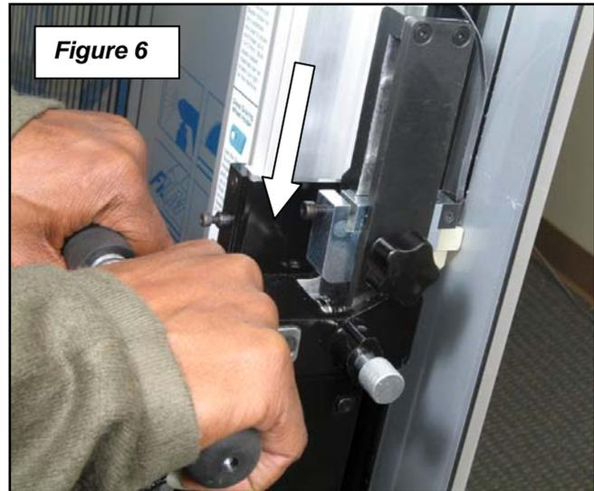
3. Unclamp the material, remove it from the FSC machine, and bend the aluminum composite sheet as desired. You may make additional V-groove cuts in the same sheet in any location or direction.
